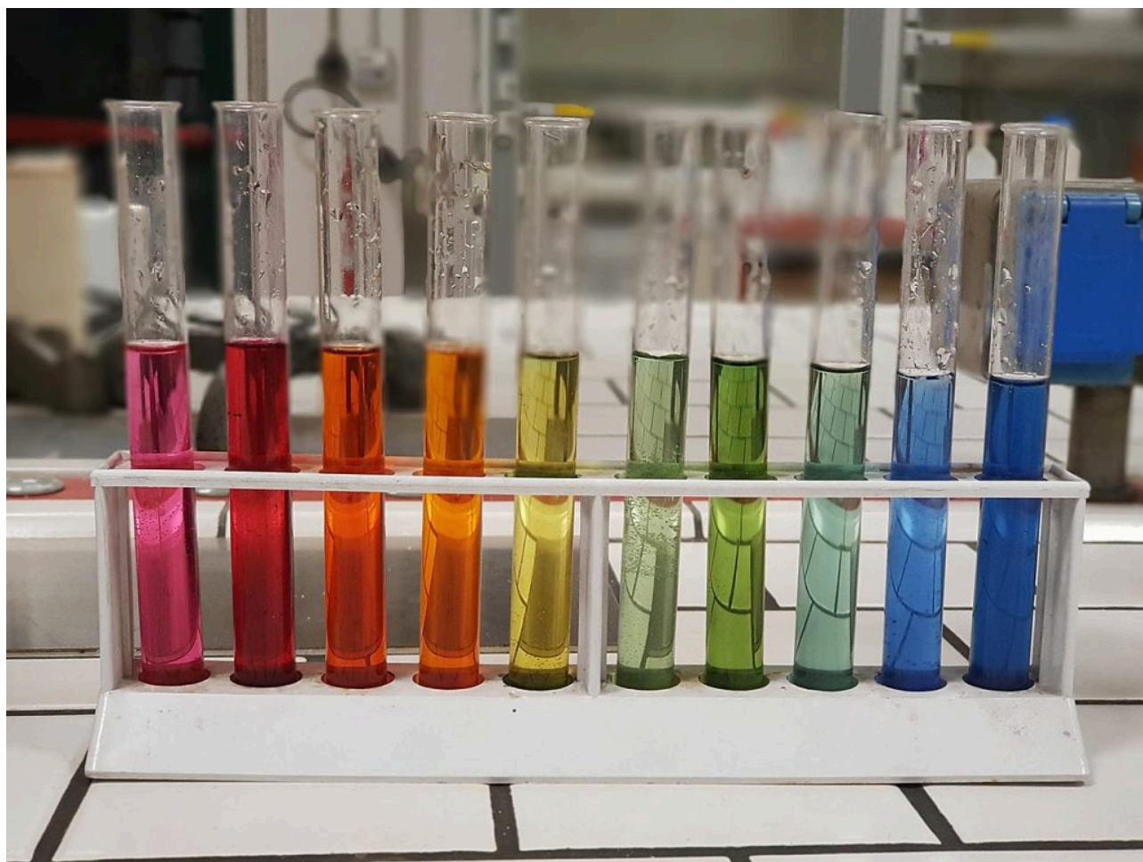
Figure 2.36. Test tubes containing solutions of pH 1–10 colored with an indicator . Image attribution: Alvy16 , PH scale 3 , CC BY 4.0
