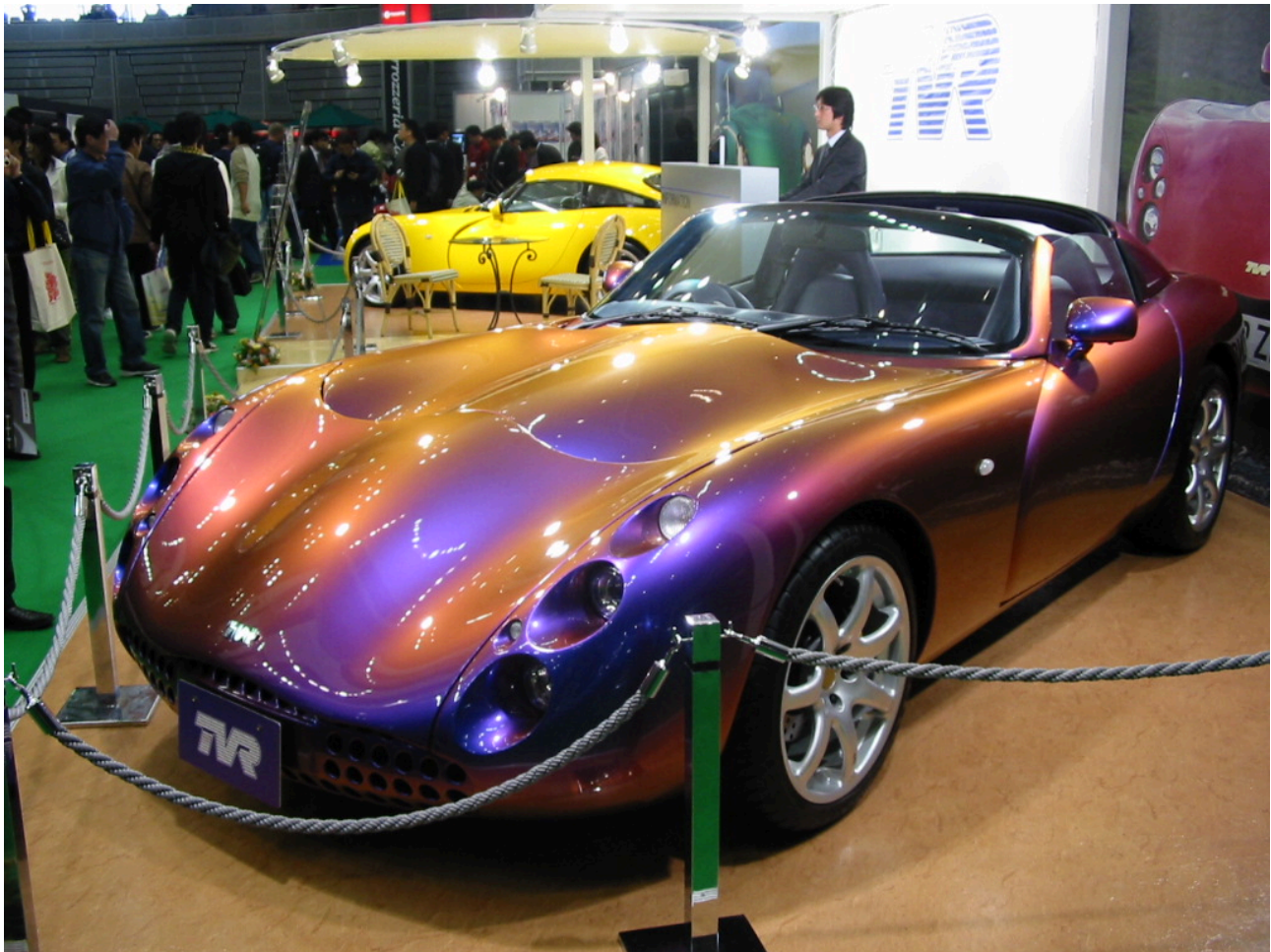
Figure 3.51. TVR Tuscan Speed Six car painted with ChromaFlair interference pigment. Image attribution: Mytho88, TVR Tuscan 01, CC BY-SA 3.0 from Wikimedia commons
