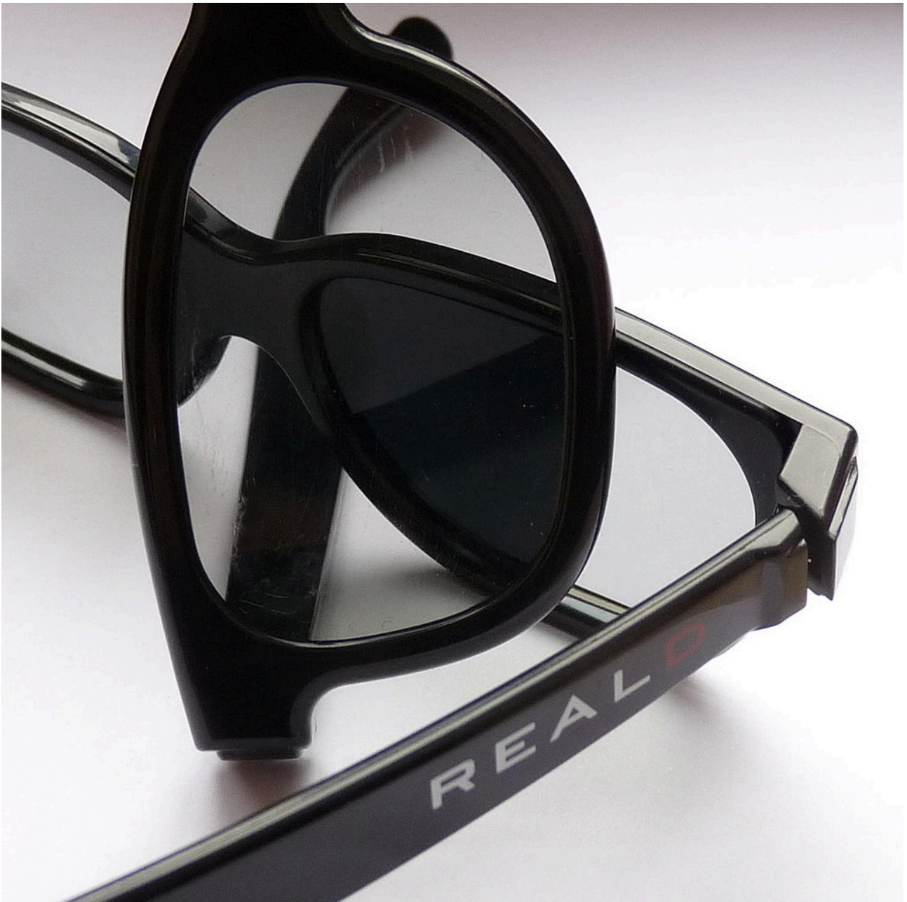
Figure 2.12. Two pairs of RealD 3D cinema glasses demonstrating polarising effect. Image attribution: Fritz Jörn at English Wikipedia, TwoRealDglassesblackening, marked as public domain, on Wikimedia Commons
