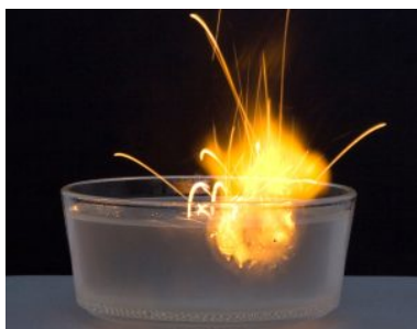
Figure 7.1.2: Metallic sodium reacts quite violently with a rather tame substance: water. The reaction often causes a small explosion! Image attribution: Metallic sodium in water © Alexandre – stock.adobe.com i
